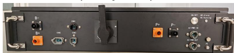
Polarity marking on high voltage control box
